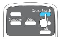
• Press the button for the source you want on the remote control. If there is more than one port for that source, press the button again to cycle through the sources.
